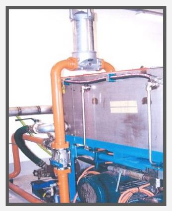
New filtration was installed to provide suitable protection from contaminants for the expanded hydraulic system.
