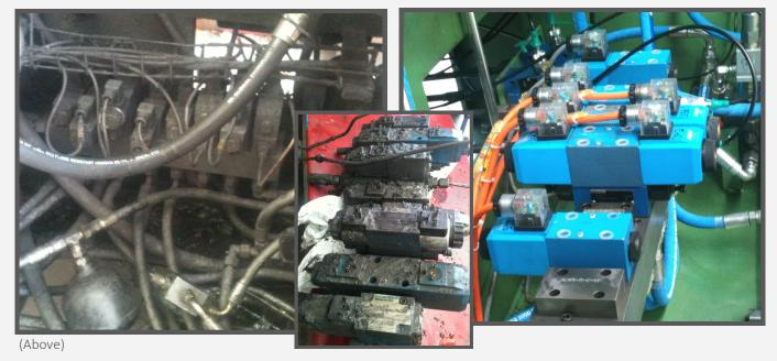
The directional control valve manifold was a sludge encrusted mess in a spaghetti jungle of hoses and wiring when it arrived at Stenmar. The finished valve bank was neatly mounted, wired, labeled and hosed.
