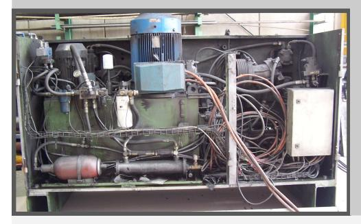
When a steel manufacturing machine had a major hydraulic failure, it resulted in nearly every component being extensively damaged.
