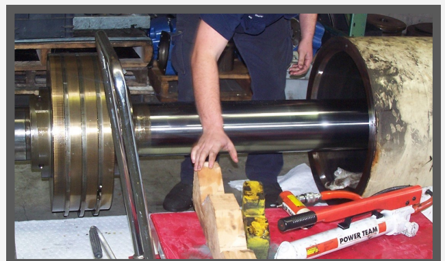
Main press ram being stripped & assessed before being comprehensively overhauled.
