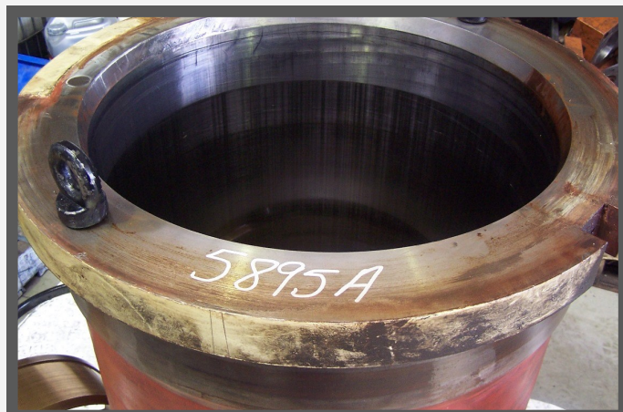
Main press ram being stripped & assessed before being comprehensively overhauled.
