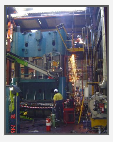
The various other cylinders were dismantled and completely overhauled in the Stenmar workshop. All wiring and cabling was renewed and a new electrical control panel built.
